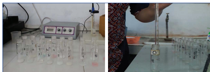
[Table/Fig-3]: A 0.25 mL in duplicate of the suspension were transferred to test tubes. [Table/Fig-4]: A 0.25 mL of 2.0 M hydrochloric acid was added to break mono fluoro phosphate ion into fluoride ion. (Images from left to right)
