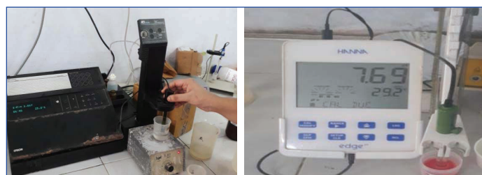
[Table/Fig-9]: Fluoride concentration was determined fluoride electrode coupled to anion analyser (Orion EA-70) was used. [Table/Fig-10]: pH of the suspension was determined using pH meter. (Images from left to right)
