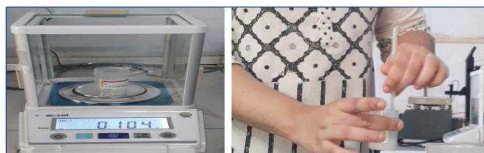
[Table/Fig-1]: A 90-110 mg of toothpaste was weighed. [Table/Fig-2]: The toothpaste was homogenised with 10 mL of distilled water. (Images from left to right)
