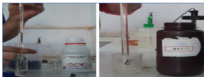
[Table/Fig-7]: Acidified solution were neutralised with 0.5 mL of 1M sodium. [Table/Fig-8]: The suspension was further neutralised with 1 mL Total ionic strength adjustment buffer II. (Images from left to right)
