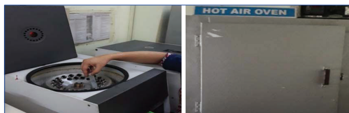
[Table/Fig-5]: Dentrifice suspension was centrifuged (10 min at 3000 g) at room temperature. [Table/Fig-6]: 0.25 mL of the supernatant, 0.25 mL of 2.0 M hydrochloric acid was added and the tubes were kept in a hot air oven for 1 hour at 45°C. (Images from left to right)
